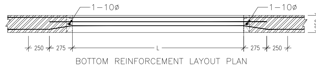
LINTEL DETAIL FOR 250 MM THICK. WALL
