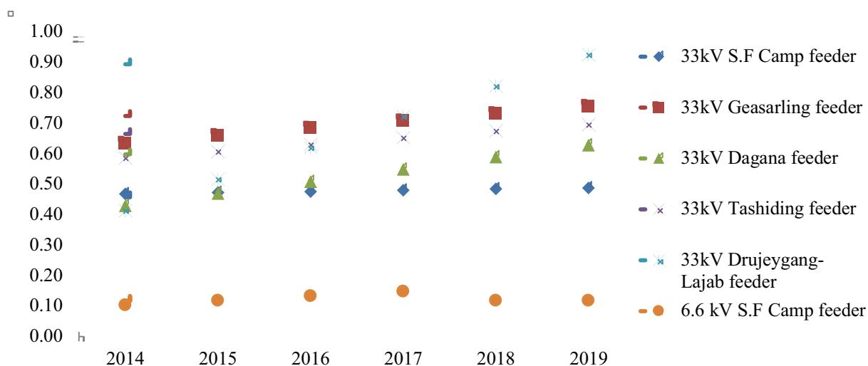
Figure 3: Feeder wise peak load
