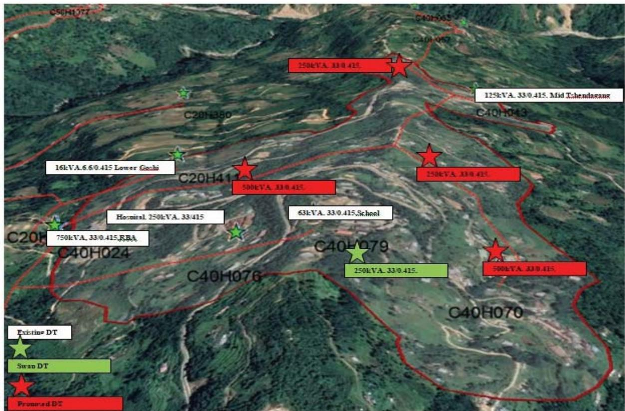
Figure 9: Proposed location the installation of additional DTs
